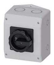
SENTRON, Switch disconnector 3LD, main switch, 3-pole, lu: 63 A, Operating power / at AC-23 A at 400 V: 22 kW, molded-plastic encapsulation for metric screw connection, 1 NC, 1 NO, rotary operating mechanism, black
